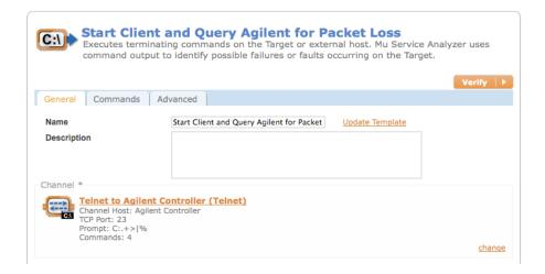
Setting up the Mu to control the Agilent N2X is a three-step process. First we must establish a Telnet session with the N2X controller. This is done through the Channel specification.
