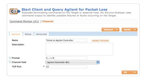
In order to navigate the login process that occurs over telnet we must enter some setup actions. We will look for the word "login:" then send the username "n2x", then wait for the response "password:" and then transmit the password for the user n2x. At this point we should expect a ">" prompt to be considered successful. The other prompt specified is "%" which becomes valid in the Tcl shell.
