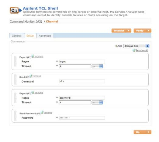
After the channel configuration is completed, the second step is to start the Tcl shell, configure the test on the Agilent N2X and begin transmitting traffic. This is done through the Setup tab that allows us to create an Expect script to interact with the channel as shown below:
